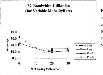
Fig 5.12 Overall network % Bandwidth utilization as a function of percentage of Routing Misbehavior
