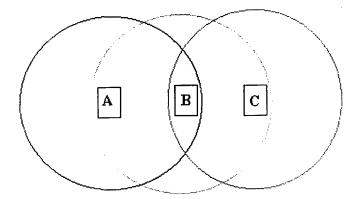
Figure 1.1 An ad hoc network of three wireless mobile hosts
