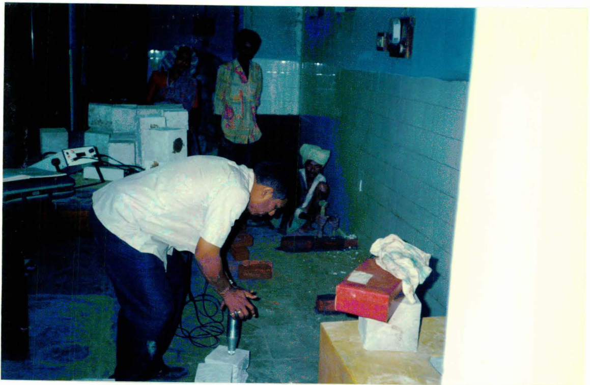
Photograph showing Schmidt hammer test being carried out to find out the rebound number.
