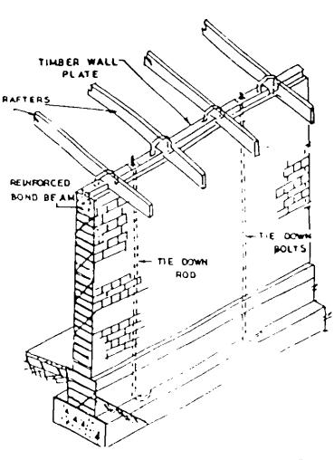
: Fixing of Walls to the Foundation Using Tie-Down Bolts Fig. E.d.
