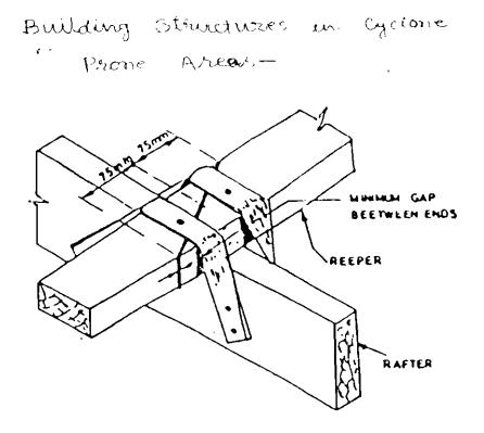
Use of Straps and Nails to Tie-down Rafter to the Top Plate
