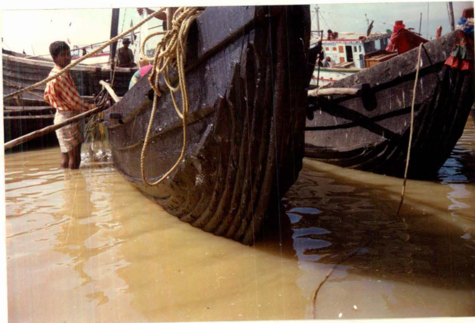
Fig.4: A patia found in North Balasore from the river Pancapara to the Subarnarekha. This reverse clinker-built boat is rare worldwide.
