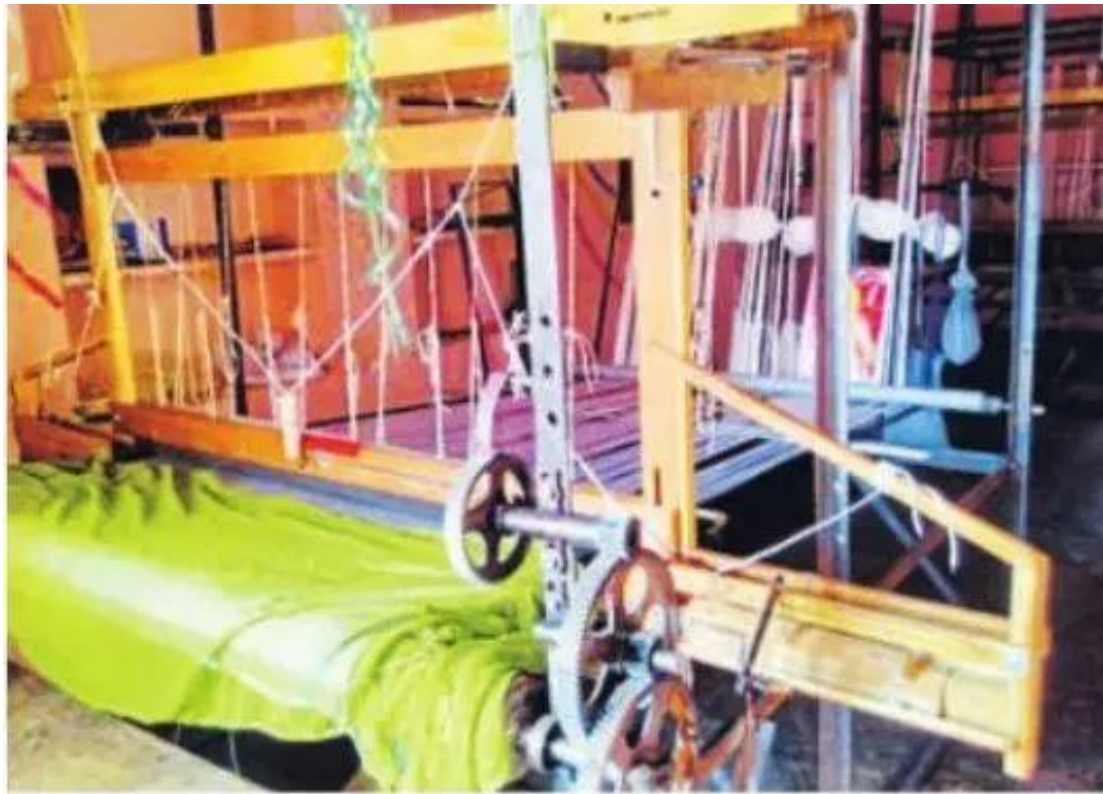
Fig. 4.7 The Traditional Weaving Machine
