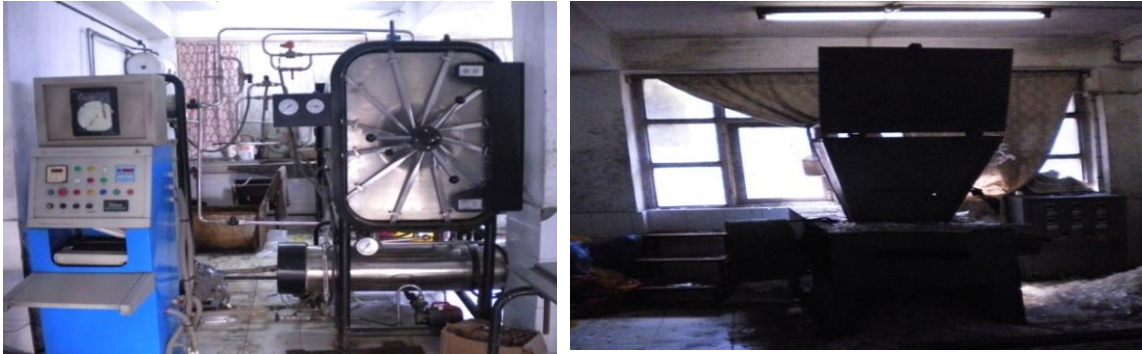
Figure: 3.18 & Fig. 3.19 - Autoclaving and Shredding unit at Tertiary care Hospital
