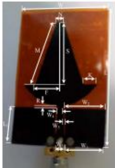
Fig. 2.5. Fabricated Prototype of the antenna presented in [33]
