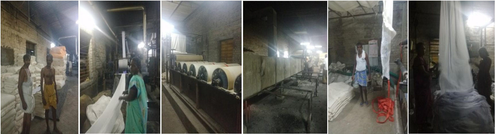
White fabric Sent through rollers to stretch length & Passed through closed furnace to stretch width Cloth Pressed and collected
