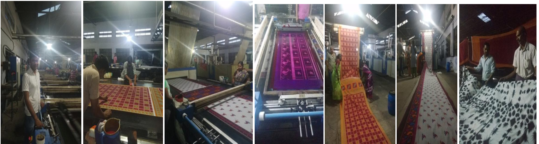
Manual checking and Automatic Screen printing on Saree cloth
