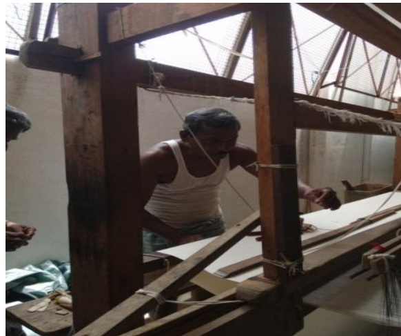
Weaving by foot pedals and hands manually
