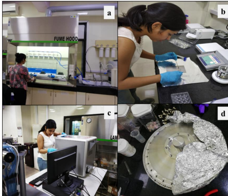
Plate 1.4 Steps involved in graphitization of sediment samples for AMS ^{14}\text{C} dating (a) ABA treatment, (b), determination of percentage carbon content in soil (filling samples in aluminium foil and), (c), graphitization of samples (d) samples after ^{14}\text{C} dating using AMS
