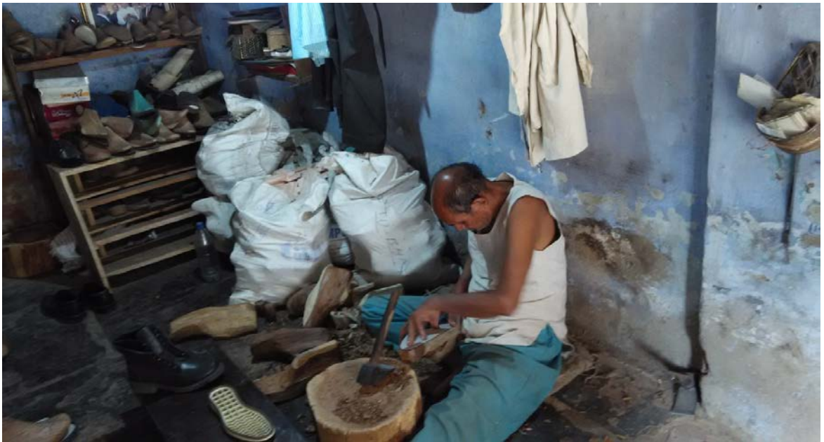
Hand made last sample making picture of a small workshop at Meera Husseni Chowk
