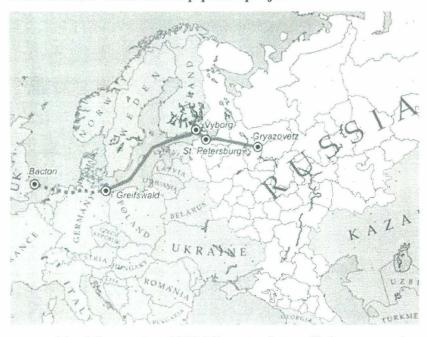
Nord Stream is a 1200-kilometre-long off-shore natural gas (from Shtockman and Yamal fields) pipeline stretching through the Baltic Sea, from Vyborg, Russia to Greifswald, Germany which is to be built by Nord Stream AG.
