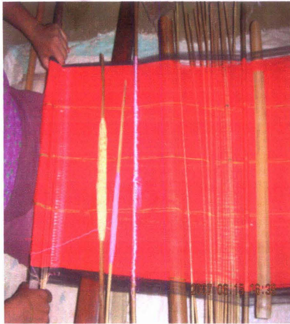
Small bamboo bars in the loom used for weaving patterns
