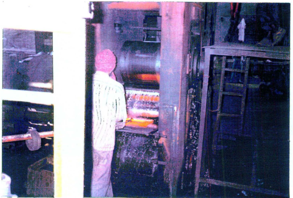
Inside the unit, cold rolling of the iron sheets
