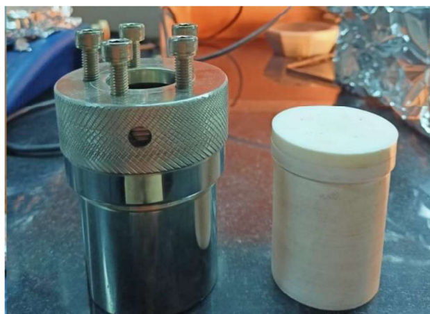
Fig 3.1 – Autoclave and Teflon container
