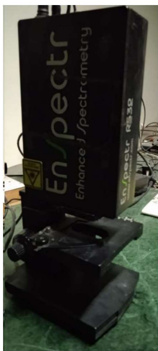
Fig 4.2 – Raman spectroscopy setup
