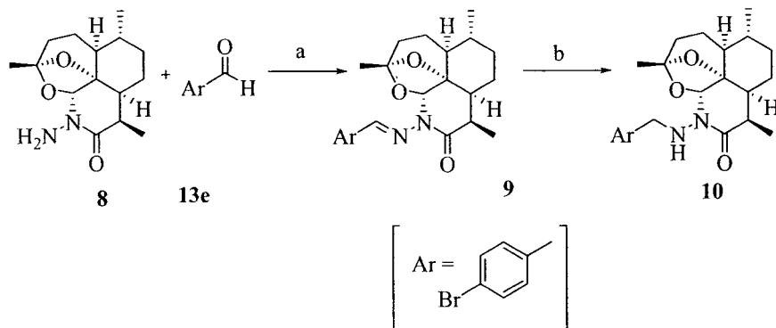
**Scheme 5.4 Reagents and conditions:** (a) Amberlyst-15, molecular sieves, dry benzene, rt, 2h; (b) NaBH<sub>4</sub>, dry benzene, 0 °C, 4 h.
