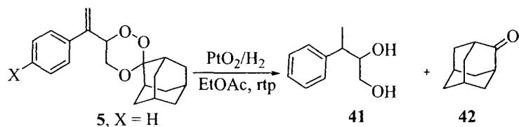
**Scheme 2.11** Catalytic hydrogenation of trioxane **5**.
