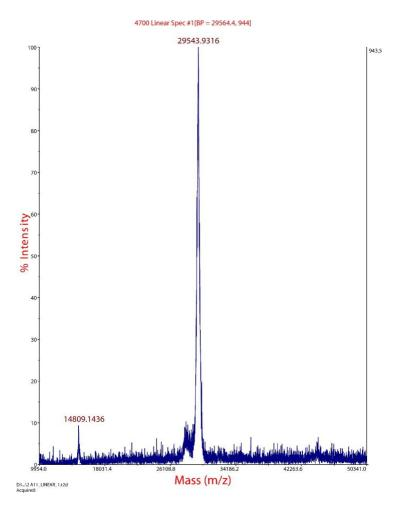
**Fig. 4.7 MALDI-TOF analysis of Rv3400.** The major peak observed at ~29543.9 Da corresponds to Rv3400.
