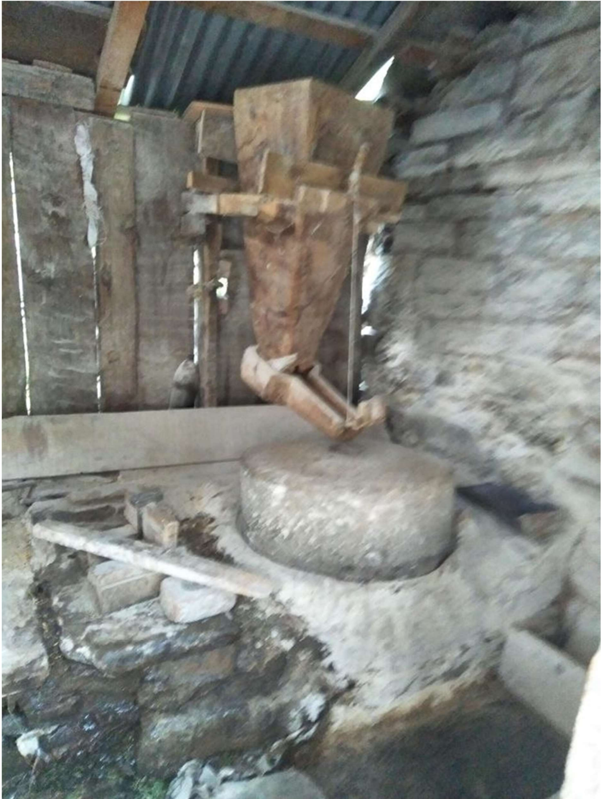
Fig 3.1 Gharaat-The Himalayan Watermill
