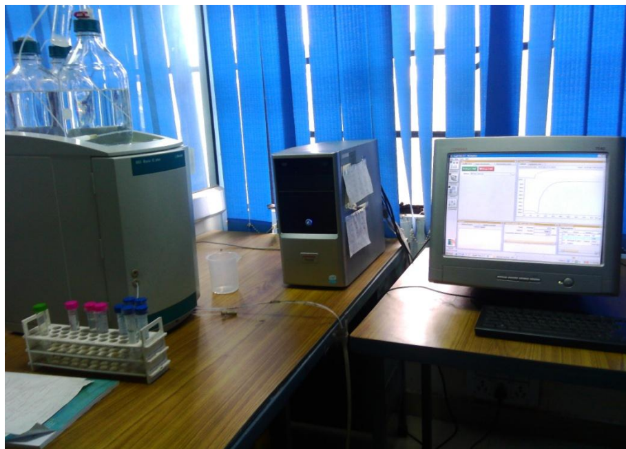
Fig.3.4. Ion Chromatography (Metrohm-883 basic plus)
