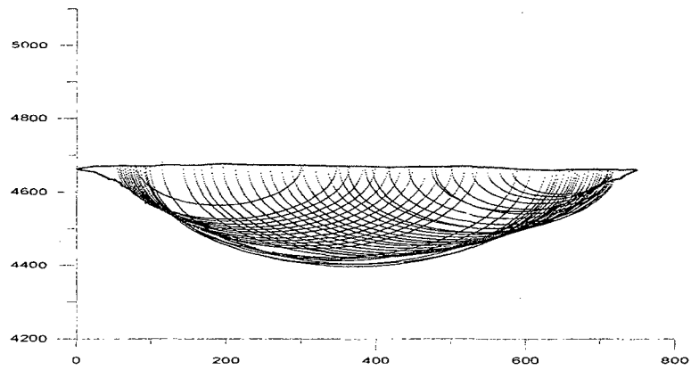
Fig. 5.14c: 2D graph of cross section-3, the vertical axis represents the depth and horizontal axis represents the length of cross section.
