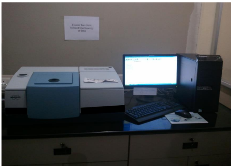
Figure 2.5. Fourier transform infra-red spectrometer.
