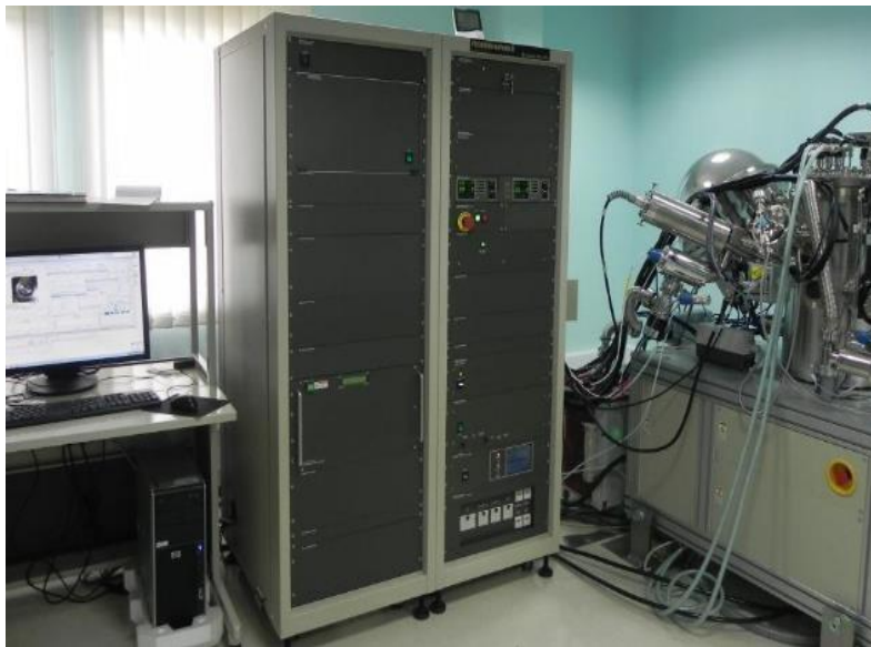
Figure 2.2 X-ray photoelectron spectrometer.
