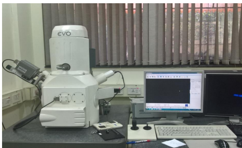
Figure 2.7. Scanning electron microscope.
