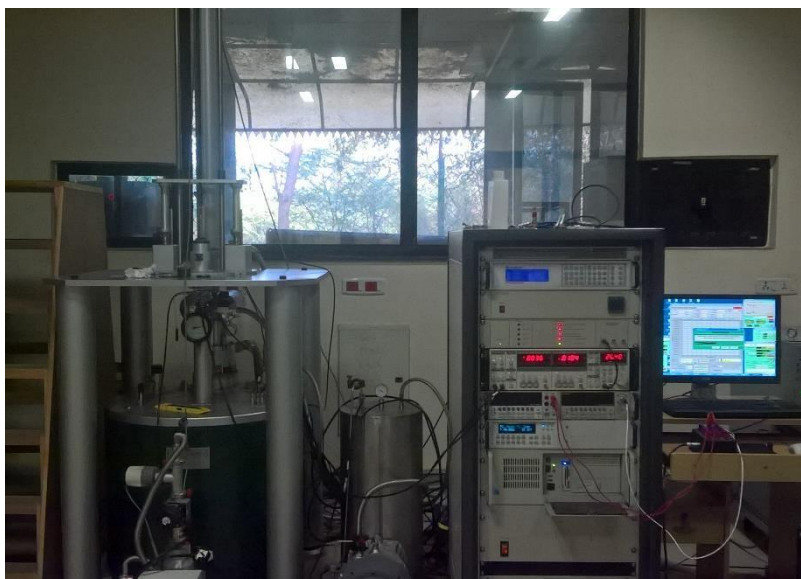
Figure 2.10. Physical properties measurement system.
