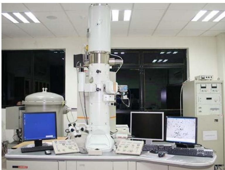
Figure 2.9. Transmission electron microscope.
