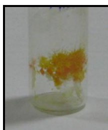
Figure 4.9 Concomitant formation of DTBHB-I and DTBHB-II . Red crystals stand for DTBHB-I and Light yellow crystals indicate DTBHB-II .
