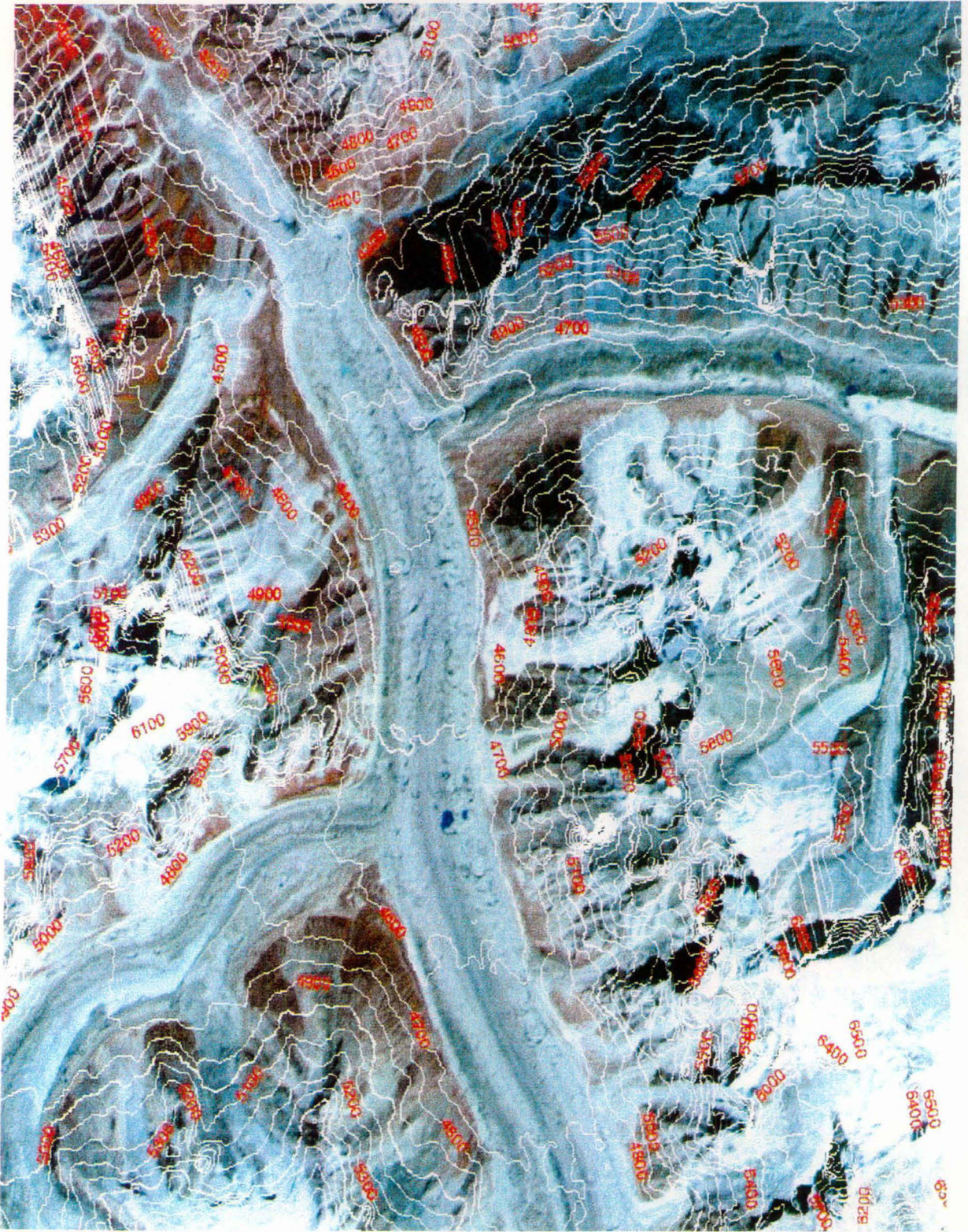
Fig. 4.2 DEM of Gangotri Basin Prepared from ASTER Stereo Image of Sept. 2001 (Source : US Geological Survey)
