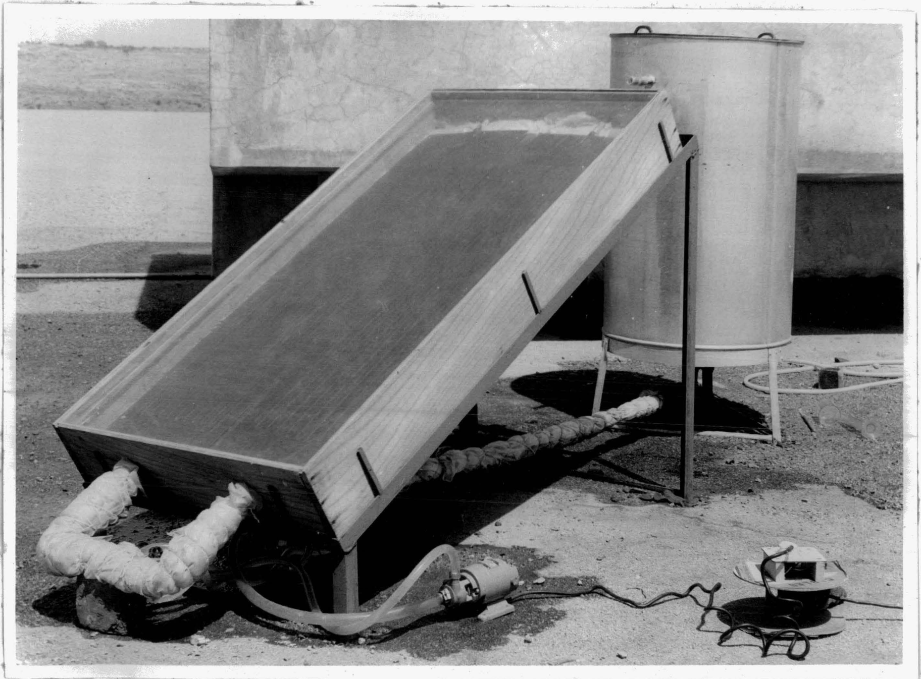
Fig.(i): CONSTRUCTED FLAT PLATE SOLAR WATER HEATER
