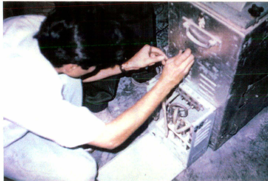
LOW VOLUME SAMPLER FOR MEASURING OTHER INDOOR AIR QUALITY PARAMETERS
