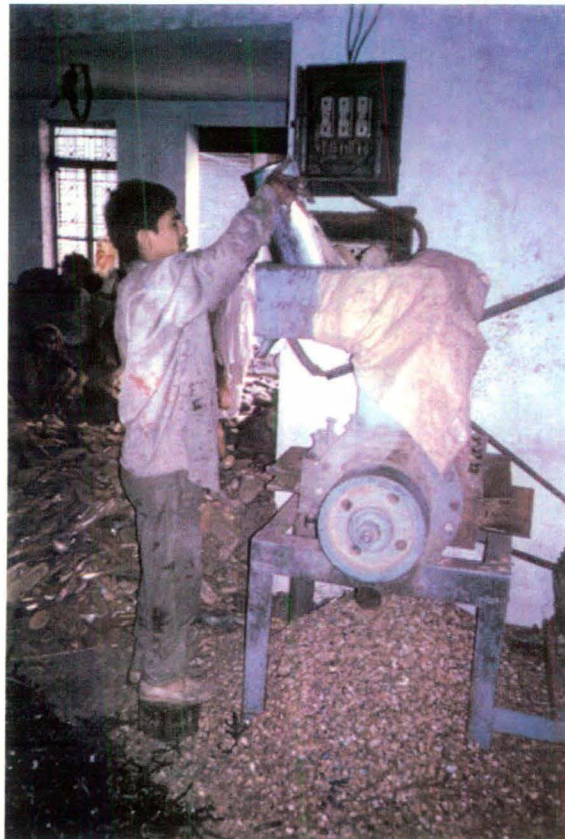
SORTED FOOTWEAR BEING GROUND FOR REPROCESSING AND CONVERSION TO SECONDS FOOTWEAR
