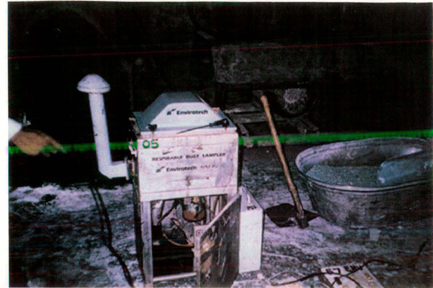
HIGH VOLUME SAMPLER FOR MEASURING DUST
