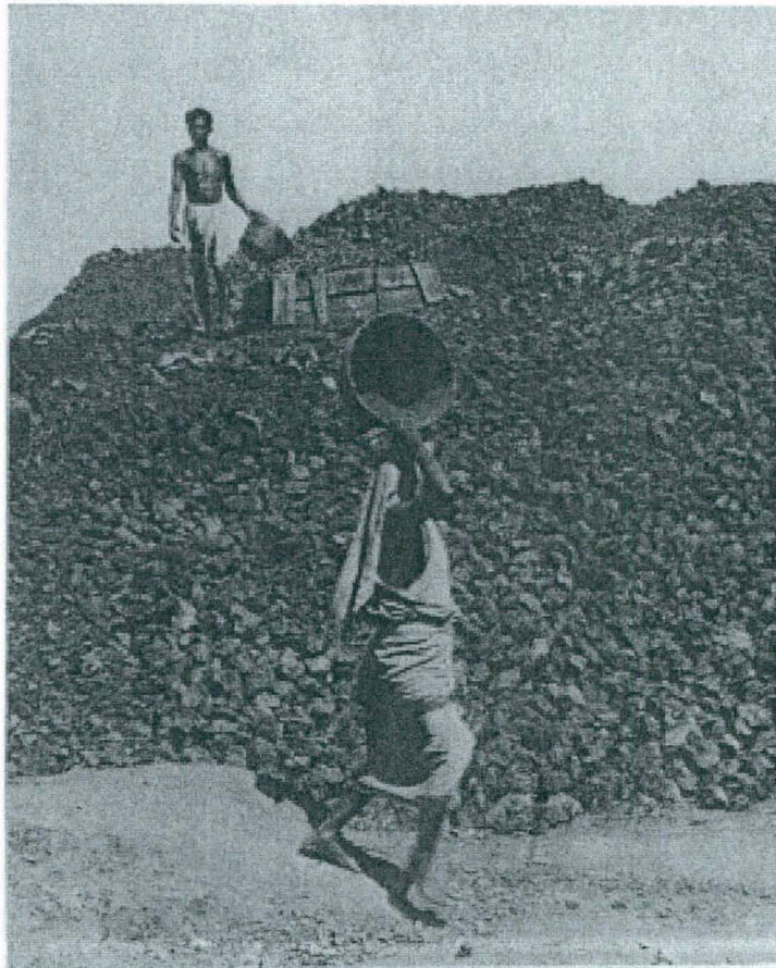
Fig.6. Mined ore is being stacked by Ho workers. The miners carry the ore in buckets and dump it in wooden boxes used as a measure for payment of wages. The stock piles are located on the level areas between tracks and mining faces.
