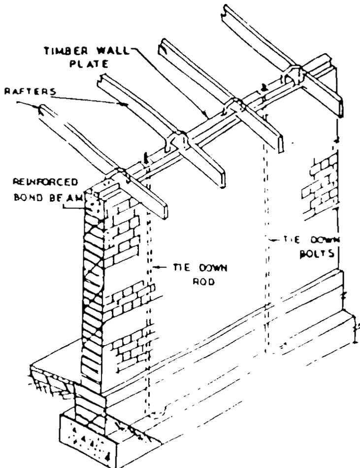
: Fixing of Walls to the Foundation Using Tie-Down Bolts
