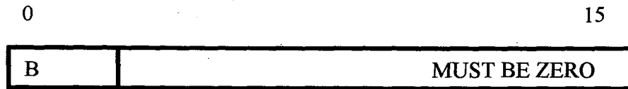
Figure-2 (The format of the 16-bit FLAGS field in a DHCP message)
