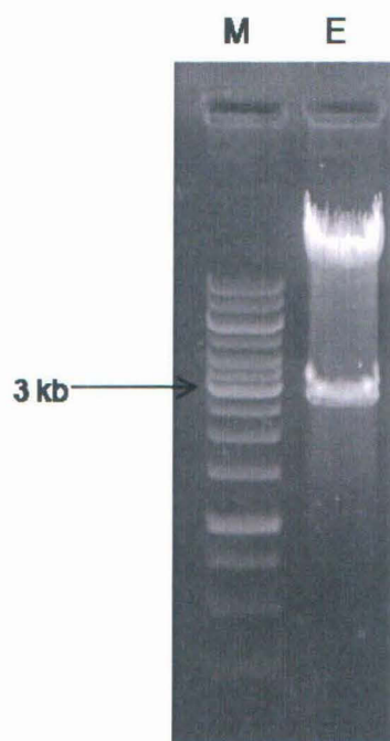
Fig 21: Restriction digestion of chitinase-pCAMBIA 1301 vector to release chitinase gene. The pCAMBIA 1301 vector was digested with HindIII to check the correct cloning of the chitinase gene in the pCAMBIA 1301 vector. A band (CaMV35S-chitinase-polyA) of ~3kb was observed in the lane E. 1.0 kb DNA ladder was loaded in the lane M.
