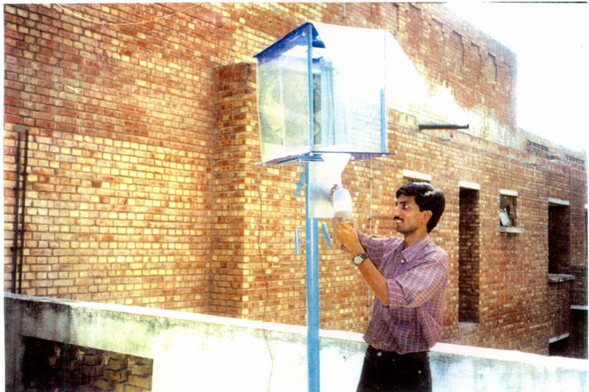
Figure 2.1: Nylon Fibre Active Fog Water Collector
