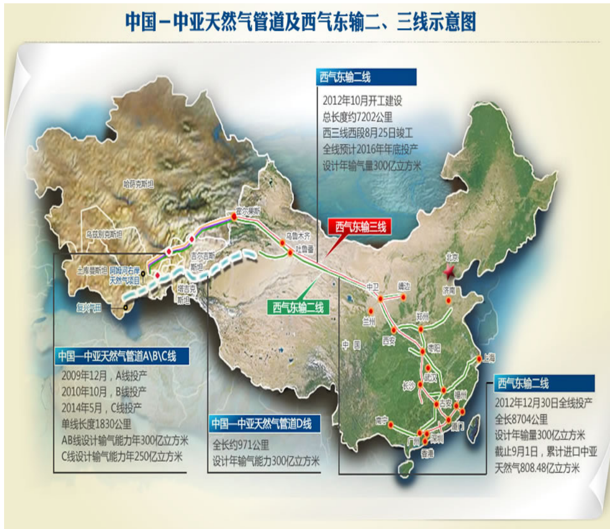
Figure 3.3 Schematic Diagram of China-Central Asia Gas Pipeline and West- East Gas Pipeline
