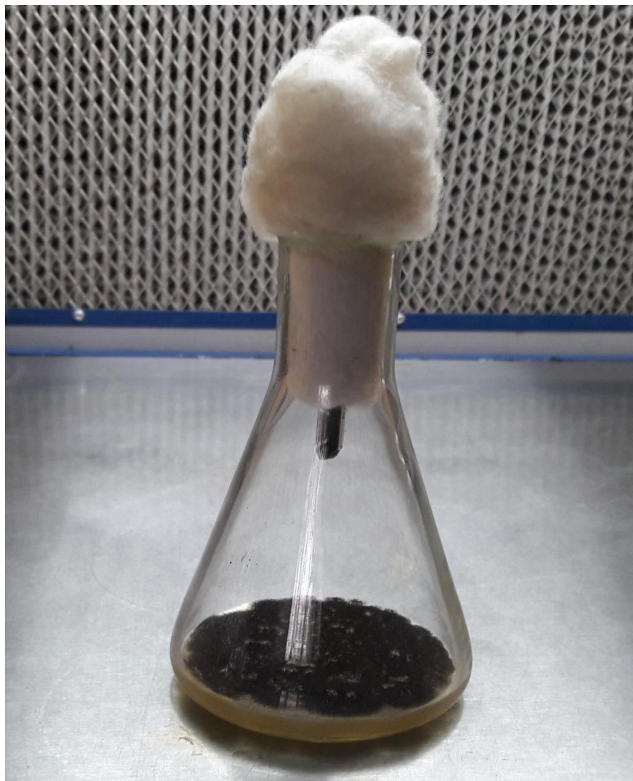
Figure 2.10: Experimental setup for passive sampling of MVOCs released from pure fungal culture
