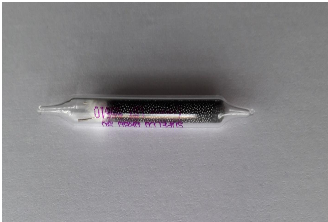
Figure 2.9: ORBO TM 90 Carboxen ® 564 charcoal tube used for sampling of MVOCs
