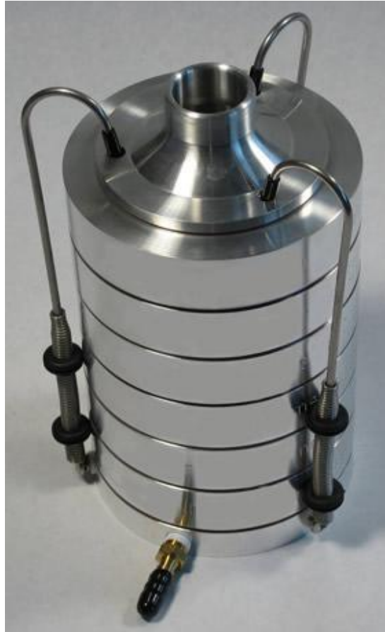
Figure 2.2: Anderson six-stage viable bioaerosol sampler
