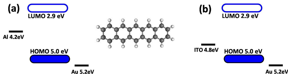
Figure 5.1: Schematic representation of energy level diagram in (a) Al/pentacene/Au and (b) ITO/pentacene/Au based two terminal devices. In the middle, optimized structure of pentacene molecule has been shown.
