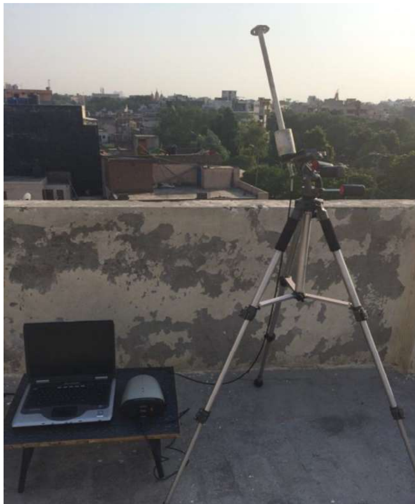
Figure 2.2. FieldSpec Spectroradiometer (ASD Inc.) used for the solar irradiance (Global and Direct) measurements.
