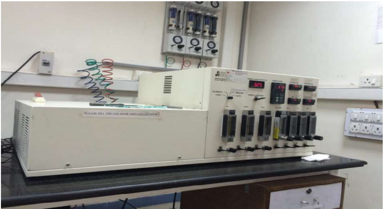
Figure 2.4. EC/OC Analyser (DRI) used for the analysis of Organic and Elemental carbon in PM 2.5 samples (Source: Central Instrumentation Facility (CIF), School of Environmental Sciences (SES), JNU, New Delhi).
