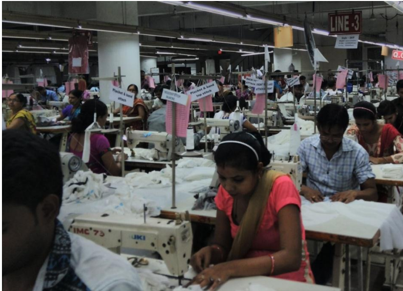
Plate No. 5 - Stitching Department (Line 3) - The stitching takes place in line with each worker sewing a particular portion of the garment
