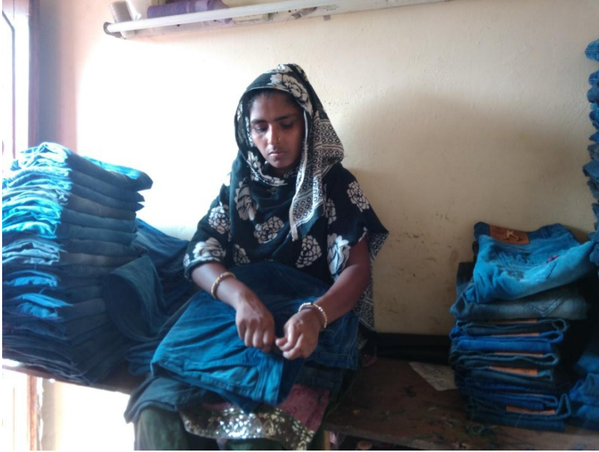
Plate No. 17 – Dhaga Cutting - (Removal of Excess Threads) of Garment by Helper. She is working without any protection has danger of inhaling tiny pieces of thread which may affect her health.
