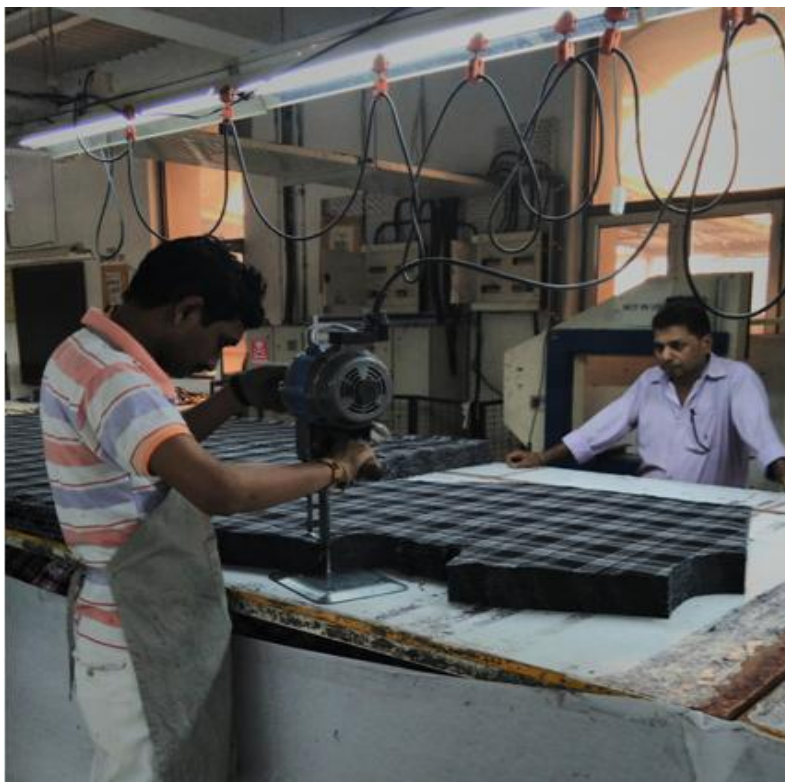
Plate No. 2 – Male Sample Cutters on Machine - The machine for sample cutting is mainly operated by male workers; it is then send to the stitching or tailoring department (go to Plate 3)
