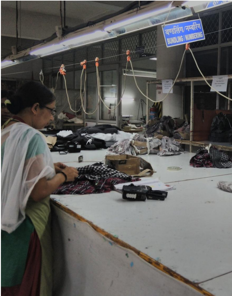
Plate No. 3 - Numbering or Bundling of Sample – After cutting every sample is denoted with a tag number, so as to keep a track of its progress or making
