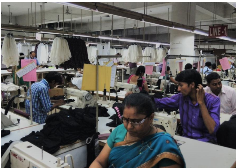
Plate No. 4 - Stitching Department – (Line 1) The stitching takes place in line with each worker sewing a particular portion of the garment
