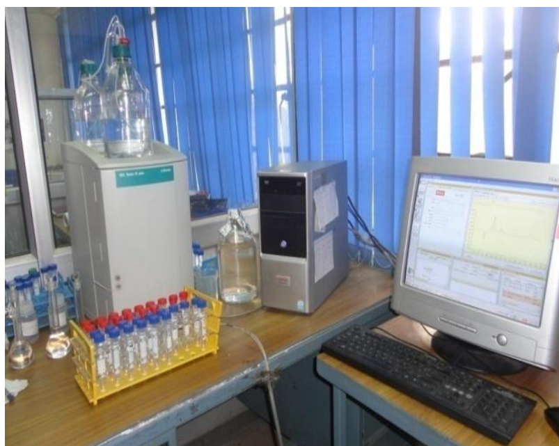
Fig. 3.3: Ion Chromatograph model Metrohm 883 used for the determination of ions in this study.
