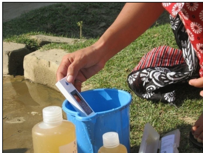
Fig. 2.13 Determination of Electrical Conductivity (EC) of Water sample from Banwas
