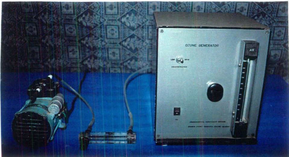
Plate 2.3: BARC Model Ozone Generator with Rotameter.
