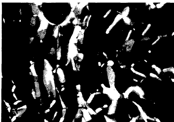
Figure 2.7: Typical texture of the ribbon phase (R) observed between crossed polarizers, on cooling from the L_\alpha phase.
