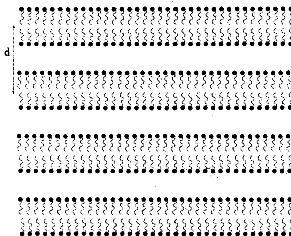
Figure 1.9: Schematic diagram of the lamellar phase which consists of bilayers stacked one above the other. d is the lamellar periodicity.
