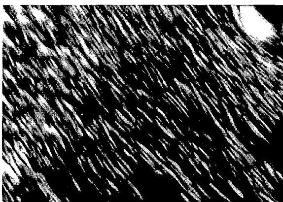
Figure 2.6: Typical texture of the lamellar phase with defects ( L_\alpha^D ) when observed between crossed polarizers at 30 °C.
