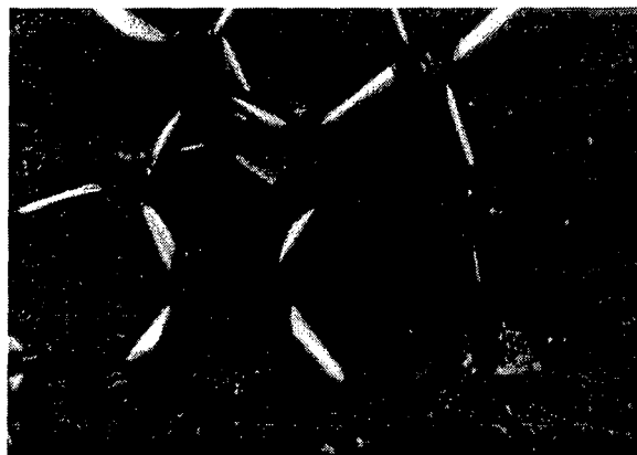
Figure 2.1: Flow birefringence of the isotropic phase of CTAB-SHN-water system ( \alpha = 0.25 ) observed between crossed polarizers on shearing at 30 °C. The birefringence observed here (indicated by the bright regions) occurs due to the flow of the sample trapped between air bubbles.
