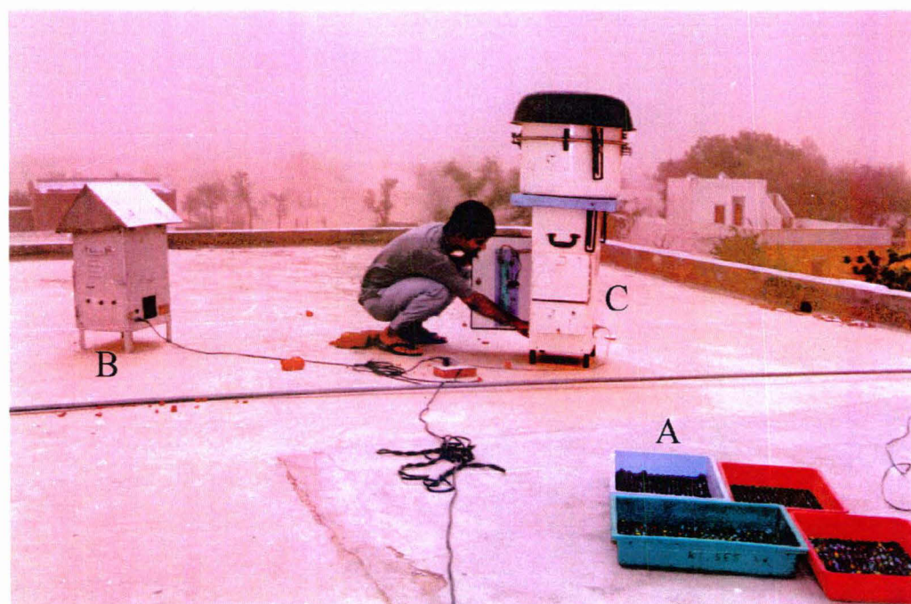
Figure 3.1 Various sampling techniques used for aerosol sample collection. (A) Trays containing marble bi-layers for free-fall collection. (B) High-volume air sampler for SPM collection. (C) High-volume air sampler for PM 10 collection.
